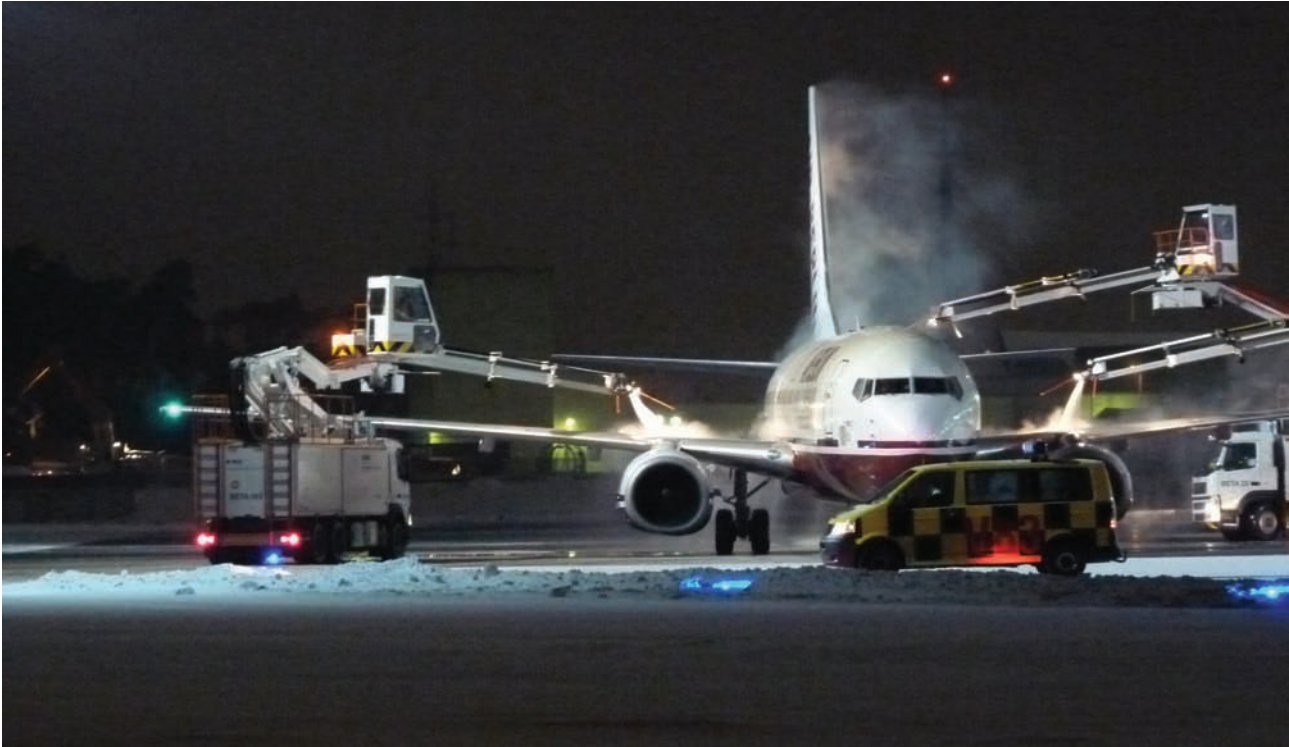
Remote de-icing positions help Frankfurt Airport to keep gates free.
